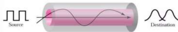
b. Multimode, graded-index
